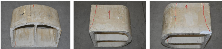
Cracked segment of lining structure (7# ~ 8#) (a)
