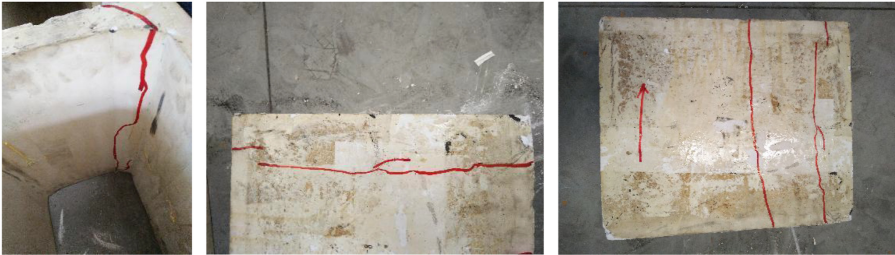
Cracked segment of lining structure (11#) (e)
