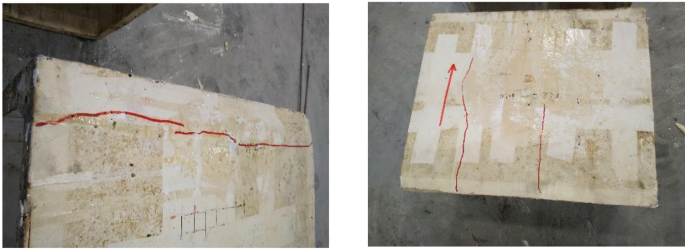
Cracked segment of lining structure (7#) (a)
