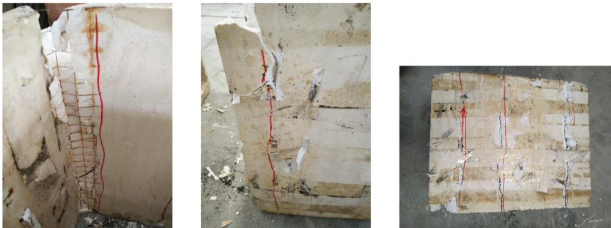
Cross-fault cracked section of lining structure (9#) (c)
