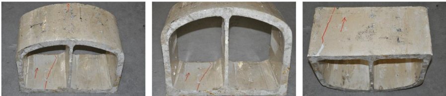
Cross-fault cracked section of lining structure (9#) (b)
