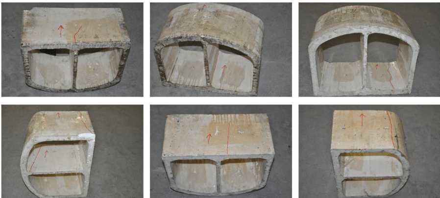
Cracked segment of lining structure (10# ~ 12#) (c)
