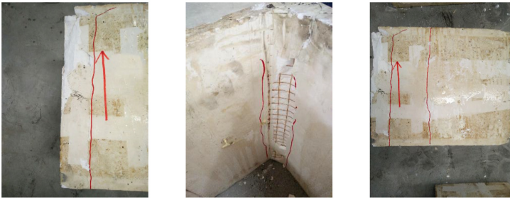
Cracked segment of lining structure (8#) (b)
