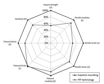
Figure 9 Comparison between mechanical properties of samples made in the injection moulding technology and samples made in the FFF technology
