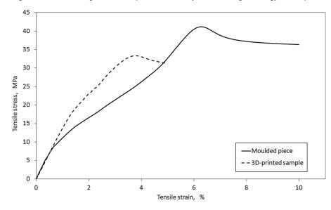
Figure 8 Sample runs during the bend test for samples made in the injection moulding technology and samples made in the FFF technology
