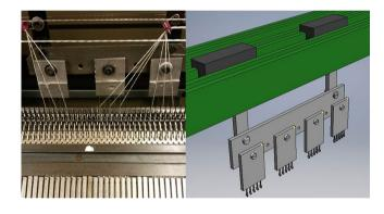
Figure 8. Warp insertion device on electronic machine, and CAD drawing of device
