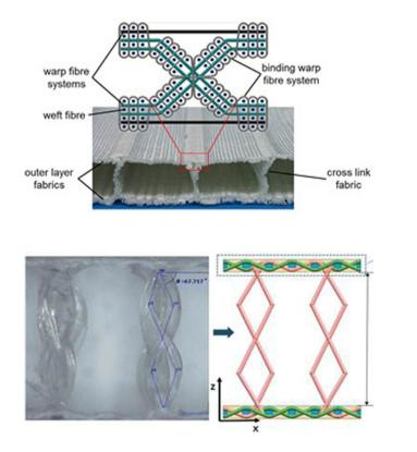
Figure 4. Structural unit of 3D woven hollow integrated sandwich composites (Liu *et al.*, 2017)
