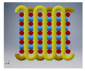
Figure 2. Side view of orthogonal woven structure bias direction for the orthogonal structure, compared to the multi-axial structures, which required much higher stress for lower strains.
