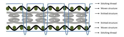
Figure 6. Schematic of a 3D stitched wovenknitted structure
