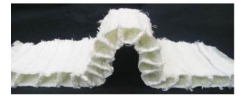
Plate 2. Flat knitted multilayer reinforced curvilinear 3D spacer fabric (Abounaim, 2011, by the kind permission of Md. Abounaim)
