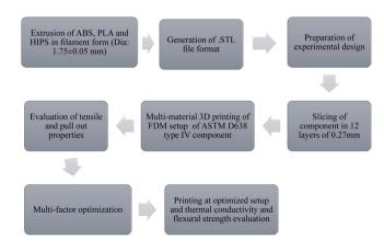
**Figure 1.** Steps involved in multi-material 3D printing etc. These properties are defined under the controlled continuous heating (endothermic reaction) and controlled continuous cooling (exothermic reaction). The endothermic reaction was carried under the heating rate of  $+10^{\circ}$ C/min from 30°C to 250°C, whereas exothermic reaction was carried under  $-10^{\circ}$ C/min from 250°C to 30°C. Figure 3 show the experimental setup of a DSC and internal configurations.
