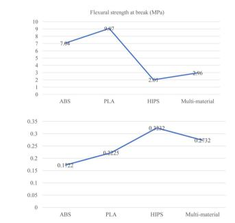
having thermal conductivity of 0.2225 W/m.K, ABS of 0.1722W/m.K and HIPS of 0.3232W/m.K. For structural applications, it requires the thermal conductivity to be desired minimum. Multi-material printing of these material resulted in thermal conductivity of 0.2732W/m.K (dt/dT= 0.814 K/s) which was lesser than HIPS material shows the utility of multi-material 3D printing.
