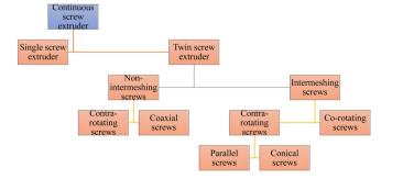
Figure 4. Classification of extrusion process
