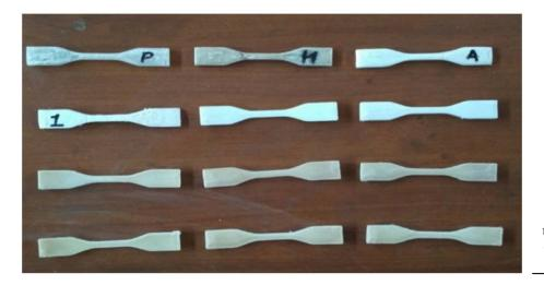
Figure 7. 3D printed multimaterial component as per ASTM D 638 type IV
