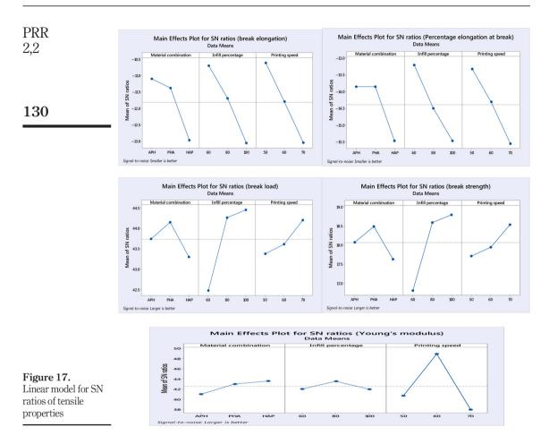
From here, it was observed that for changes in the break elongation as tensile properties of 3DP multi-material component, material combination contributed 25.41 per cent, infill percentage contributed 35.31 per cent and printing speed was contributed maximum as 37.0 per cent. The residual error was observed 2.25 per cent that shows the good control over the processing of components (Table III).
