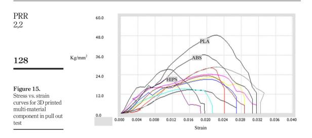
resulting in more uniformity. The tensile strength for experiment number 3 (Table II) was observed as maximum, the interlayer connectivity of ABS, PLA and HIPS thermoplastic was observed as better (Figure 16). For experiment number 1, where tensile strength was resulted in the minimum values the micrographs highlights that the layer connectivity in this case in not uniform so less strength was attained (Figure 16).
