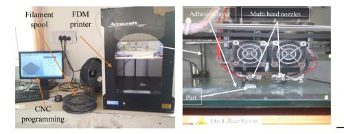
Figure 6. Commercial FDM setup
