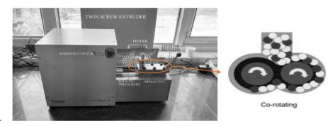
Figure 5. Photographic view of the experimental setup for extrusion of feedstock filaments
