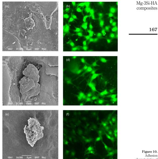
**Notes:** (a and b) Mg-3Si; (c and d) Mg-3Si-5HA; (e and f) Mg-3Si-10HA composite surface
