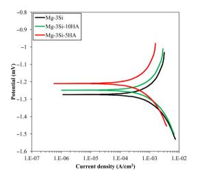
Figure 7. Potentiodynamic polarization curves of Mg-3Si, Mg-3Si-5HA and Mg-3Si-10HA composites in SBF (Ringer's Solution) at (37 ± 1)°C
