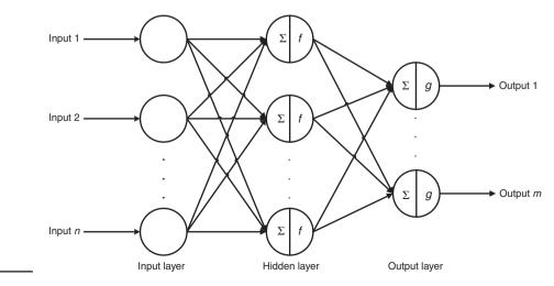
Figure 1. ANN structure output layer is represented as  $O = (O_1, O_2, ..., O_m)^T$ . Suppose the weight between the input layer and the hidden layer is  $w_{ij}$ , the weight between the hidden layer and the output layer is  $w_{jk}$ , and the input  $I_i$  is known, then, the output of hidden layer and the output layer can be calculated by the following equation:
