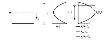
Figure 1. Concrete wall heated on both sides, cross-section (left), temperature distribution (center) and distribution of concrete strength (right)
