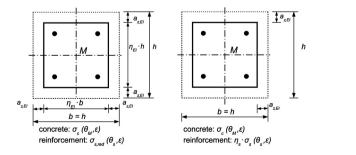
Figure 2. Square cross-section for the Zone Method by Cyllok and Achenbach (left) and proposal for the extended Zone Method (right)
