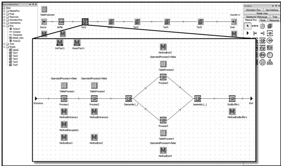
Figure 5. Screenshot plant simulation: line assembly simulation system
