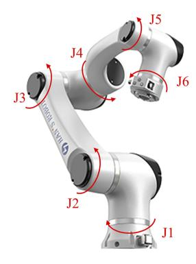
Figure 3. Structure of the simulation 6 DOF robot
