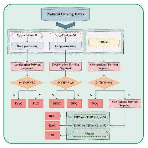
Figure 7 Schematic diagram of acceleration and deceleration segment label
