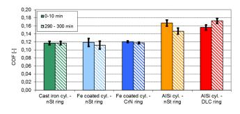
Note: Mean values for the first and last 10 min of the tribometer test
