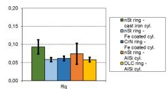
Figure 7 Cylinder liner running in for different material pairings (measured with RIC)
