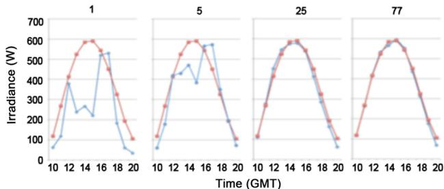
**Figure 6.** Profiles of hourly mean solar irradiance for April 30, 2009 in the Northeast Region, for a set of 1, 5, 25 and 77 stations (respectively from left to right) taken at random
