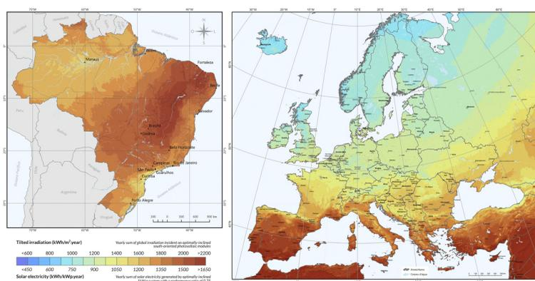
**Note:** Also shown the equivalent yearly sum of solar electricity generated by optimally inclined 1kWp system with a performance ratio of 0.75 (unit: kWh/kWp.year)
