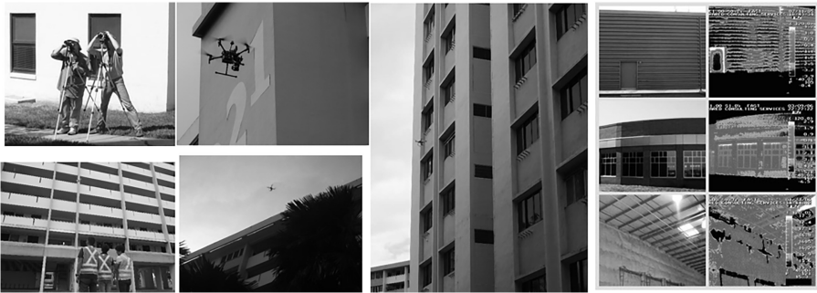
Plate 2. Stage 1 - visual investigation for 100% of the façade surface area
