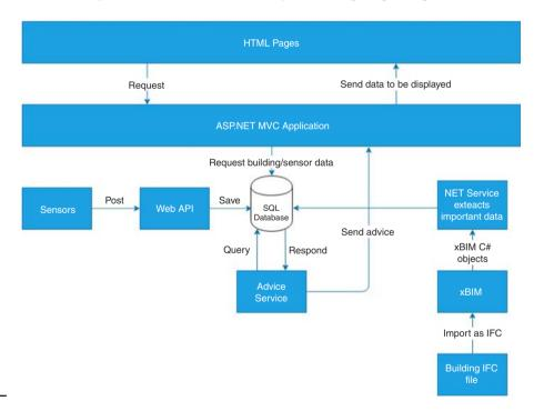
**Figure 4.** Platform system architecture
