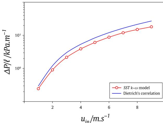
**Figure 7.** Comparison of the Dietrich's pressure drop correlation ([Dietrich, 2012](#)) and the numerically simulated data from the tetraikadecahedron PCL model with  $\varepsilon = 92\%$
