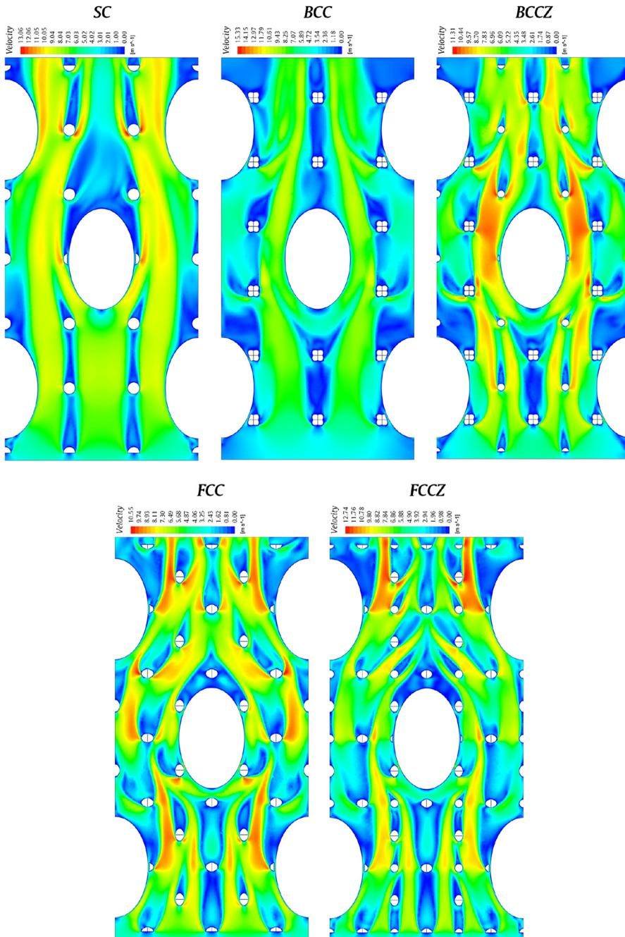
**Figure 12.** Local distribution of the velocity (in the middle  $xy$ -plane) for PCLs at  $\epsilon = 92\%$ ,  $Re_{D_h} = 3000$
