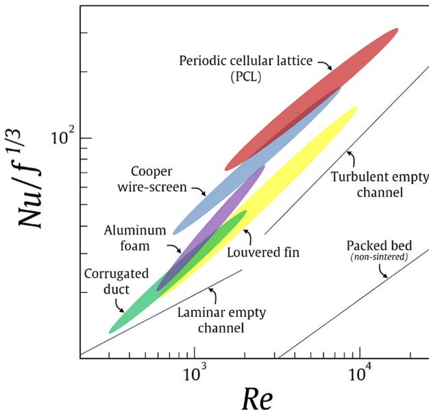
**Figure 2.** THP comparisons of various heat transfer enhancement media with selected data from [Kim \*et al.\* \(2005\)](#)
