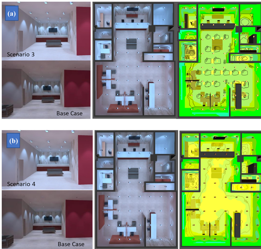
Figure 7. A comparison of the basic case simulation results against the third scenario (3a) and the fourth scenario (3b) (a) Utilizing 100% pure sunlight light and 35% artificial LED light throughout eight hours of daylight (PL 100%-AL 35%) (b) Utilizing 4 h at night time with 0% pure sun light and 100% LED artificial light (PL 0%-AL 100%)
