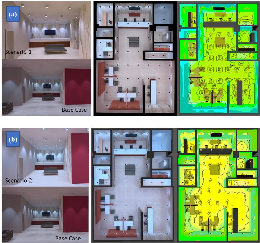
Figure 5. A comparison of the basic case simulation results against the first and second scenarios (a) Utilizing solely the HLS (PL100%- AL 0%) (b) Utilizing 100% pure sunlight and 100% LED illumination (PL 100%- AL 100%)
