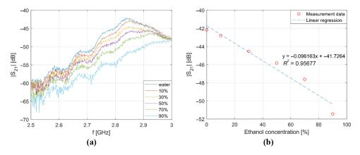
**Figure 7** The transmittance (|S21|) of the second, ring resonator for the frequency range from 2 GHz to 3.2 GHz in a function of the various volumetric concentration of ethanol in deionized water (a) and the changes of the |S21| parameter for different concentrations of ethanol at f = 2.57 GHz (b)
