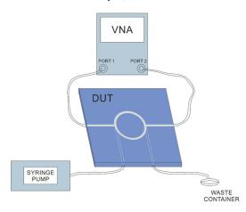
low ethanol concentrations with the R-square coefficient of 0.957 and the mean sensitivity at the level of 0.96 dB per each 10 per cent of the additional volumetric concentration of ethanol. What is more, good detection/resolution properties were obtained for frequencies ranging from 2.75 to 2.84 GHz.
