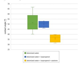
**Figure 3** A boxplot with the contact angle as a function of different types of cleaning
