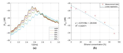
dielectric losses of the DI water around this frequency. The main principle of operation of the described microwave sensor was the shift in resonance frequency for various liquids introduced to the microchannel. The solution of the different ethanol concentrations in deionized water was introduced as a test sample because of the high difference between the dielectric constant of DI water and ethanol.
