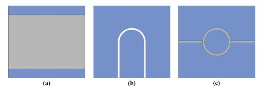
The microchannel was placed in two inner layers of the substrate (layers 2 and 3, Figure 2b). The microwave circuit was deposited on the upper layer of the substrate with the use of the ink-jet printer. The ground plane was deposited on the bottom of the module, and this time, because of cost savings, a fast version of the screen printing method was used (layer 1). Furthermore, each layer includes pads for the clamp edge-launch SMA connectors.
