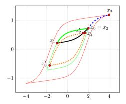
Figure 3. Reversal on a symmetrical minor loop ( $x_m = 2$ ) at x =-1 and extension to the major ( $x_m = 4$ ) loop for  $a_0 = 1.75$  and  $A_0 = 0.05$
