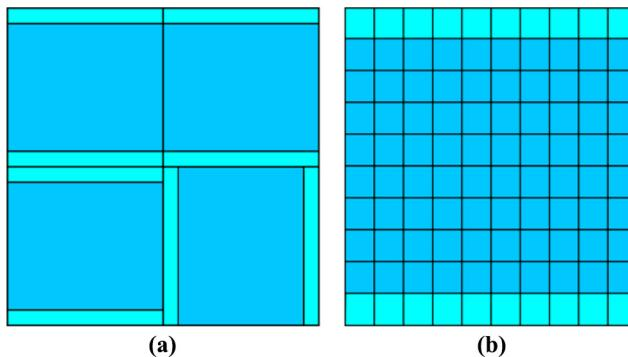
**Notes:** (a) Cross-sectional distribution in the entire four-part core. A lighter color corresponds to the value  $\kappa = 5.69$  and a darker color corresponds to the value  $\kappa = 6.39$ ; (b) projection of a 3D coarse mesh within one part of a multipart core
