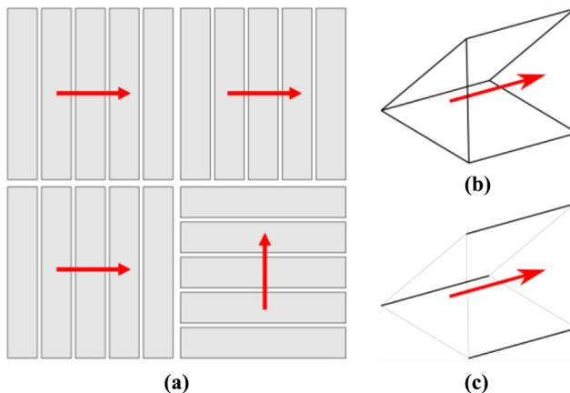
**Notes:** (a) Cross section of a laminated core. The red arrows represent the anisotropy vector for each of the four parts of the core; (b) A finite element with nine edges that are either parallel or perpendicular to the anisotropy vector (red arrow); (c) A finite element without edges to which redundant degrees of freedom are attached
