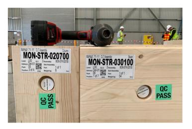
Figure 2. "Picking list" of steel components with matched tracking tag ID numbers
