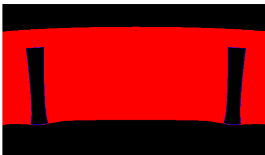
Figure A12 Equivalent Dyneema local lateral deflection representing local-buckling condition
