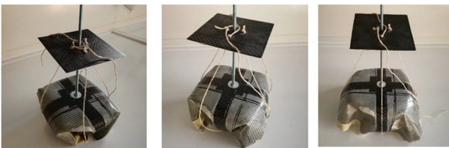
Figure A4 Possible dome deployable sequence as an example – upper plate moving outward tensioning cables and opening envelope
