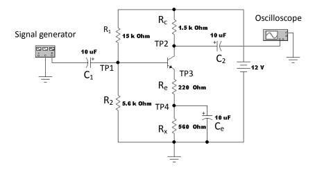
Figure 3 Prototype ORL experiment
