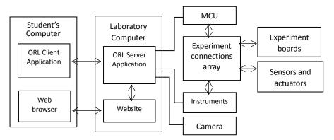
Figure 1 The ORL system architecture
