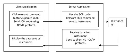
Figure 2 Instrument control architecture of the ORL system
