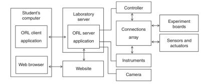
**Figure 6.** The ORL system architecture
