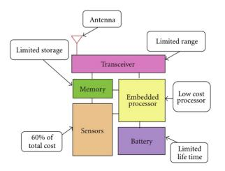
Figure 1. Wireless sensor node block diagram [1].
