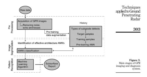
In the first segment, a preprocessing procedure has the task to: reduce noise; eliminate the undesired presence of the ground surface echo; and compensate for electromagnetic propagation losses [11,59].
